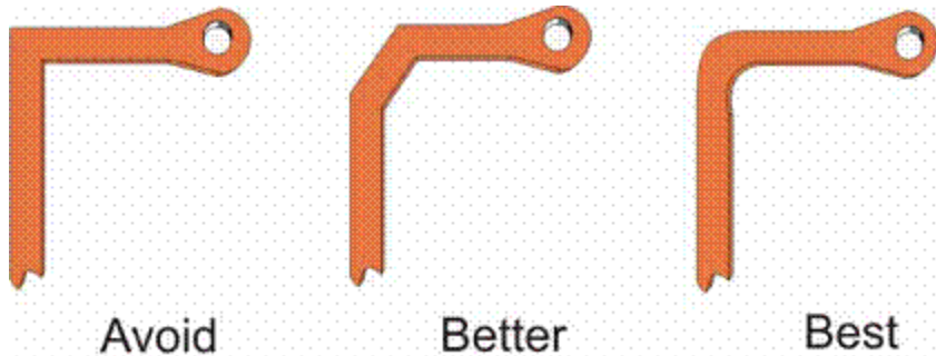
Figure 6 Routing options for flex circuit trace corners. Avoid sharp corners if possible. A radius is best as it provides a smooth transition and mitigates potential issues related to stress risers.
